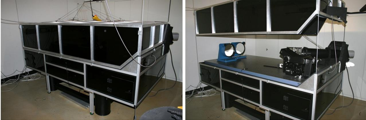
Figure 1: Left panel: The figure shows an external view of an CAFE spectrograph. The instrument is housed in a thermal isolated cabinet. Right panel: The figure shows a view of an CAFE spectrograph with the cabinet opened. The internal optical elements can be watched on the optical bench. The upper size is as straight as a die to avoid any small apertures that can break the thermal isolation. Because of that, the upper part has to be lift up with the help of a tackle.
