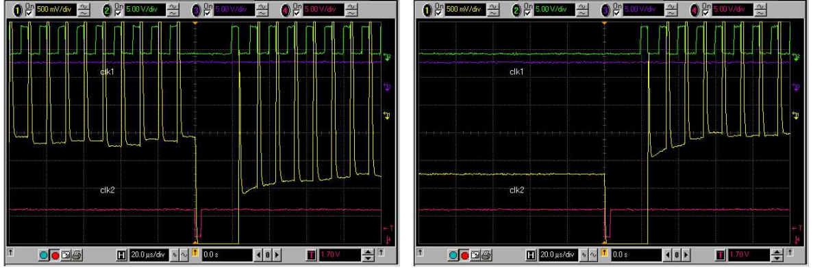
Figure 3.2: The left hand panel shows the drift in the video signal after reset and the right hand one displays it after integration. The clock signal (CLK1) is plotted with green color, the output signal of the video amplifier with yellow, and the frame synchronization signal (FSYNC) with magenta.
