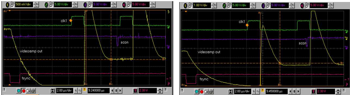
Figure 3.1: The left hand panel displays the normal triggering of the video signal conversion of the first pixel in the FPA and the right hand one the triggering with delay. The clock signal (CLK1) is plotted with green color, the output signal of the video amplifier with yellow, the start signal of the sampling (SCON) with purple, and the frame synchronization signal (FSYNC) with magenta.
